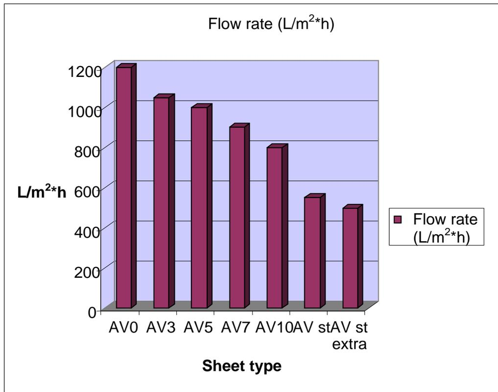
For an optimal filtration process it is recommendable to always filter with consistent flow rates, thus increasing in a progressive manner the pressure exerted: the **ENARTIS Filtra AV** range in fact has a very high mechanical resistance, capable of absorbing greater pressure differences than other common filtration sheets.
