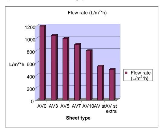
For an optimal filtration process it is recommendable to always filter with consistent flow rates, thus increasing in a progressive manner the pressure exerted: the **ENARTIS Filtra AV** range in fact has a very high mechanical resistance, capable of absorbing greater pressure differences than other common filtration sheets.
