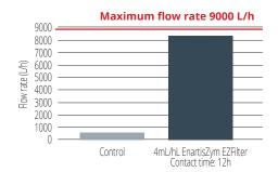
\* Must rich in colloids from Macabeo grapes. Filtration with crossflow filter with ceramic membrane and maximum flow rate of 9000L/h. In the control wine, the flow rate rapidly decreases to 500L/h. In the must treated for 12 hours with EnartisZym EZFilter, the flow rate remains constant at 8500L/h.
