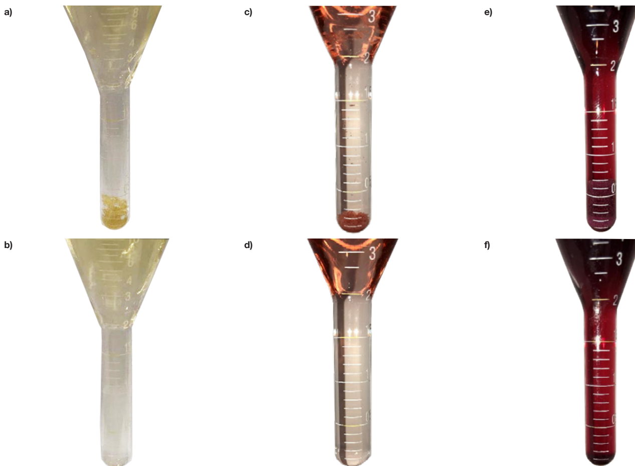
Figure 2. Comparison of untreated (top images) and KPA-treated (bottom images) samples after three months' storage. a) White wine control (untreated) sample after three months' storage (t3). b) KPA-treated white wine sample three months post-treatment (t3). c) Rosé wine control (untreated) sample after three months' storage (t3). d) KPA-treated rosé wine sample three months post-treatment (t3). e) Red wine control (untreated) sample after three months' storage (t3). f) KPA-treated red wine sample three months' post-treatment (t3).
