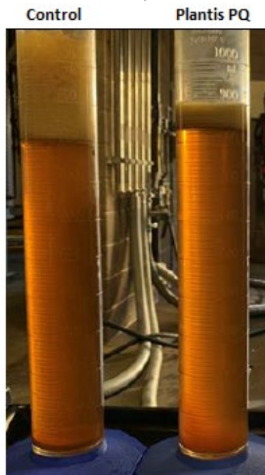
Impact of Plantis PQ (10 g/hL) on the formation of flees compared to a control with no fining agent added. Note the compaction of the floating lees cake. This leads to improved yields and better clarification.
