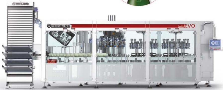
Feeding, dispensing and application of sparkling wines capsules with double centring system: orientation of the bottle (embossed logo on glass, screen print, sleeve and glass mould seaming) and capsule, both with cameras managed by SNIPER vision system.
