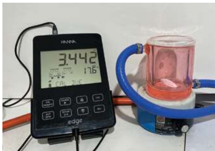
FIGURE 1: A Hanna Instrument Edge pH, Conductivity and Dissolved Oxygen meter is used with a Chemglass stirred cell to do a conductivity test to determine the stability of a rosé wine in the lab at Tamanend Wine.
