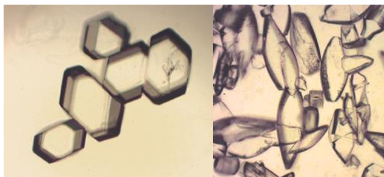
Figure 3. Typical crystal shapes of CaT (left) and KHT (right).
