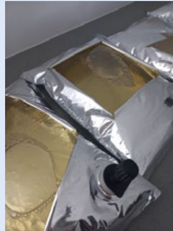
Figure 1: Headspace varies significantly from one BiB to another. This leads to a high variability in quality and shelf life of the wine within the same batch.
