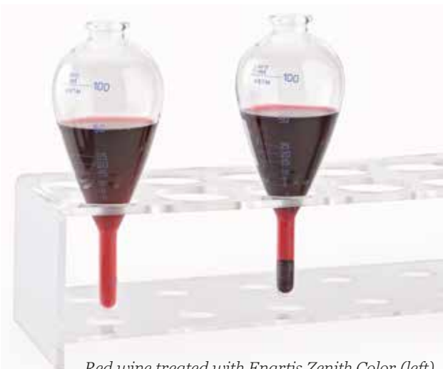
Red wine treated with Enartis Zenith Color (left) versus untreated colour and tartrate unstable red wine (right).
